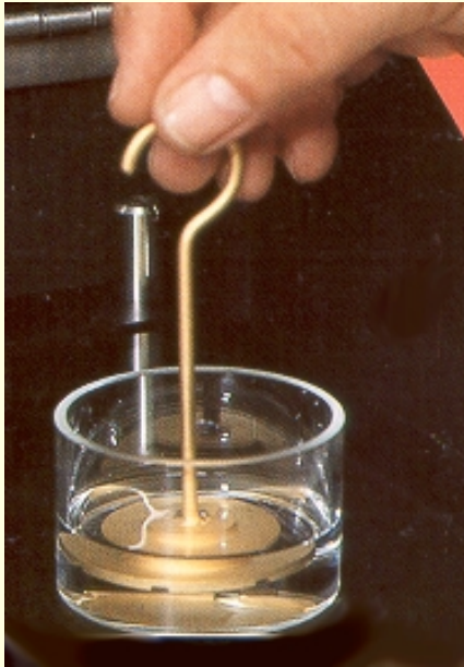
Quartz cell and gold reflector with defined path length (e.g. 0.2 mm)
