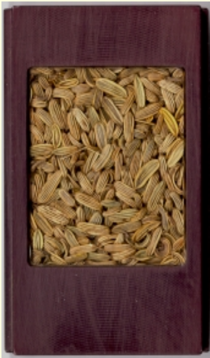
Diffuse reflection measurements in a moving sample cup with quartz window, 51 x 64 mm
